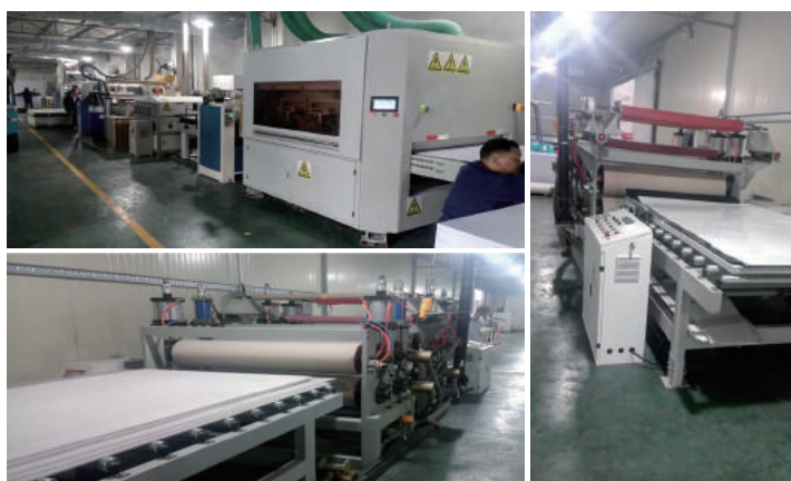
In-house PUR glue laminating production line
